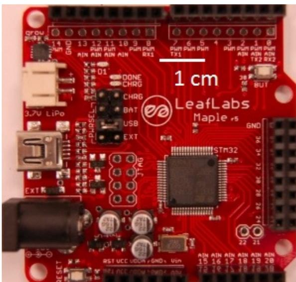
**Figure 16: The Leaflabs Maple Rev 5 microcontroller board used for the portable magnetic tweezers device.**
