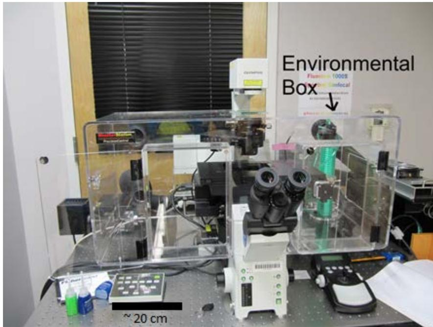
**Figure 9: Confocal microscope in the NRI / MCDB Microscopy Facility at UCSB. The microscope is outfitted with an environmental control box which places limits on the size and shape of any device interfaced with the microscope.**
