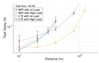
Fig. 8: Task delay over WiFi and LTE with varying distance of the UAV from the Base Station for task of burst size 50 KB every second. The measurement are taken in two different external traffic regimes of no load and high load.
