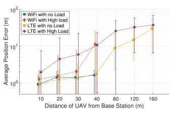
Fig. 5: Average position error and variance as a function of distance between the UAV and the base station for different communication technologies. The measurements are taken in no load and high load (8 nodes 6 Mbps each) conditions.
