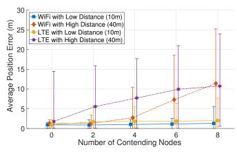
Fig. 4: Average position error and variation range for different communication technologies and protocols with respect to varying number of contending nodes. Each node is transmitting 6 Mbps data traffic.
