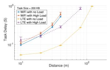
Fig. 9: Task delay over WiFi and LTE with varying distance of the UAV from the Base Station for task of burst size 200 KB every second. The measurement are taken in two different external traffic regimes of no load and high load
