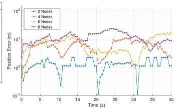
Fig. 3: Temporal evolution of position error based on the telemetry emitted by the UAV over WiFi with TCP in an urban environment with buildings. Each external node transmits traffic with rate 6 Mbps. The UAV navigates on a rectangular trajectory where the access point is at the center.
