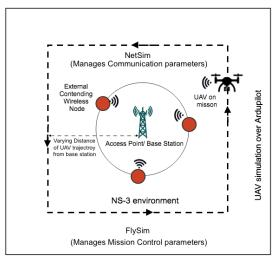
Fig. 2: Simulation setup: the UAV follows a predefined trajectory, whereas external nodes are fixed and disposed in a circle centered on the AP or eNodeB.
