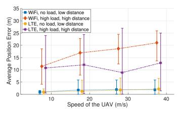
Fig. 6: Variation of Average position error with the speed of the UAV in different network load conditions over LTE and WiFi.
