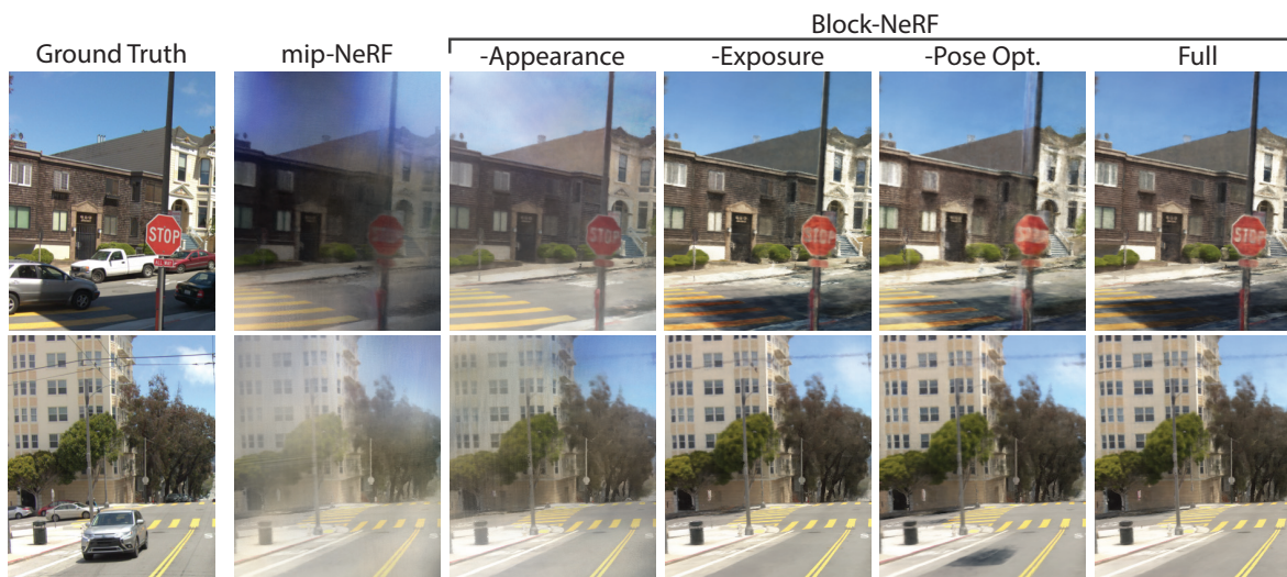
Figure 5.7: Model ablation results on multi segment data. Appearance embeddings help the network avoid adding cloudy geometry to explain away changes in the environment like weather and lighting. Removing exposure slightly decreases the accuracy. The pose optimization helps sharpen the results and removes ghosting from repeated objects, as observed with the telephone pole in the first row.
