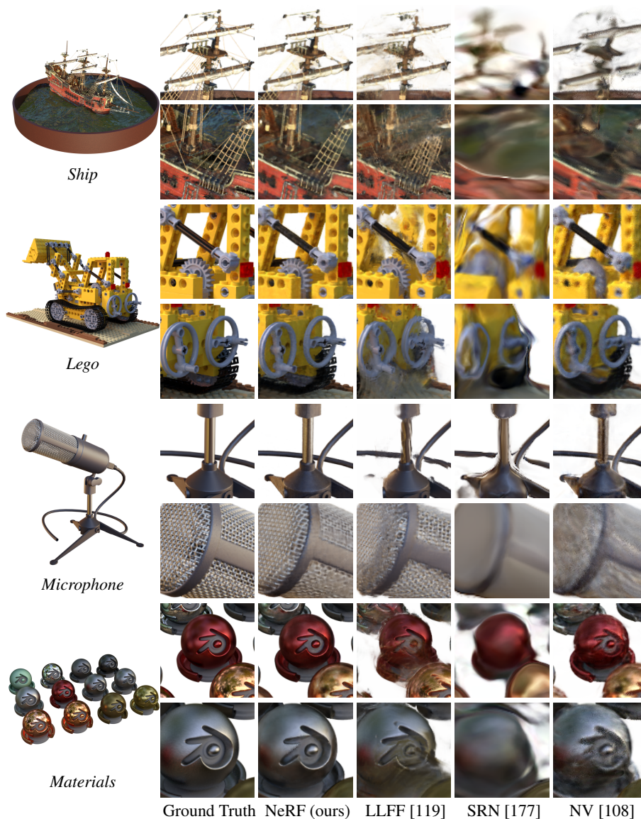
Figure 2.5: Comparisons on test-set views for scenes from our new synthetic dataset generated with a physically-based renderer. Our method is able to recover fine details in both geometry and appearance, such as Ship 's rigging, Lego 's gear and treads, Microphone 's shiny stand and mesh grille, and Material 's non-Lambertian reflectance. LLFF exhibits banding artifacts on the Microphone stand and Material 's object edges and ghosting artifacts in Ship 's mast and inside the Lego object. SRN produces blurry and distorted renderings in every case. Neural Volumes cannot capture the details on the Microphone 's grille or Lego 's gears, and it completely fails to recover the geometry of Ship 's rigging.
