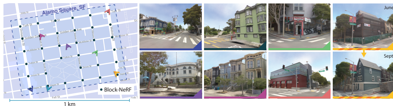
Figure 5.1: Block-NeRF is a method that enables large-scale scene reconstruction by representing the environment using multiple compact NeRFs that each fit into memory. At inference time, Block-NeRF seamlessly combines renderings of the relevant NeRFs for the given area. In this example, we reconstruct the Alamo Square neighborhood in San Francisco using data collected over 3 months. Block-NeRF can update individual blocks of the environment without retraining on the entire scene, as demonstrated by the construction on the right. Video results can be found on the project website waymo.com/research/block-nerf .
