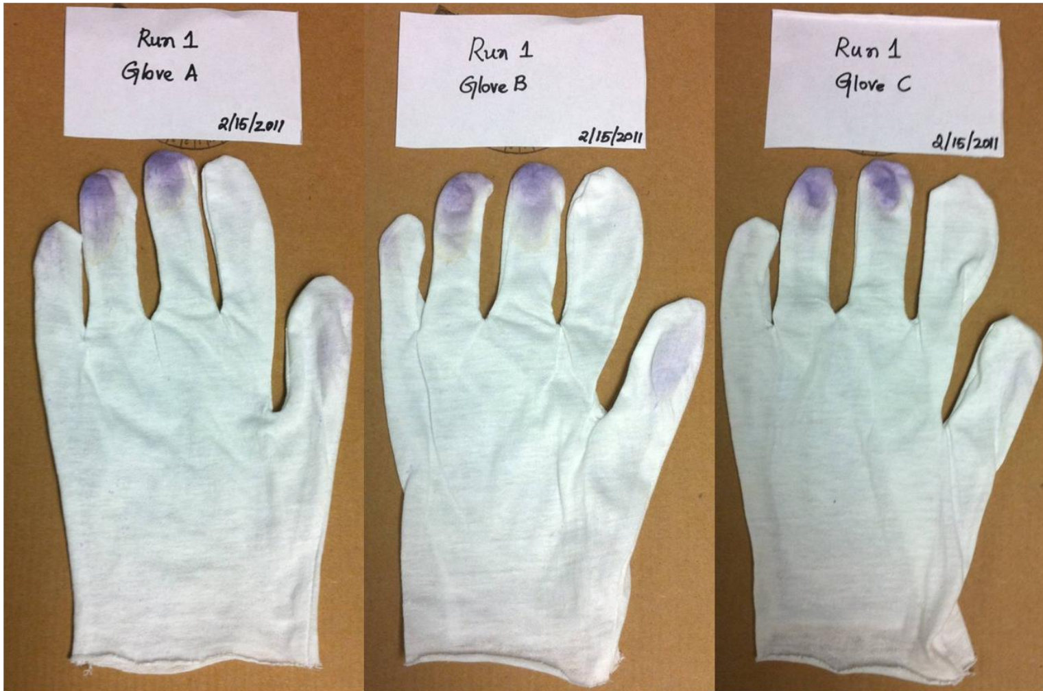
Figure 4.7: Cotton Gloves Show Indicator Dye (Contact) on Fingers After “Run 1” Pass on Turf Using the BCTU
