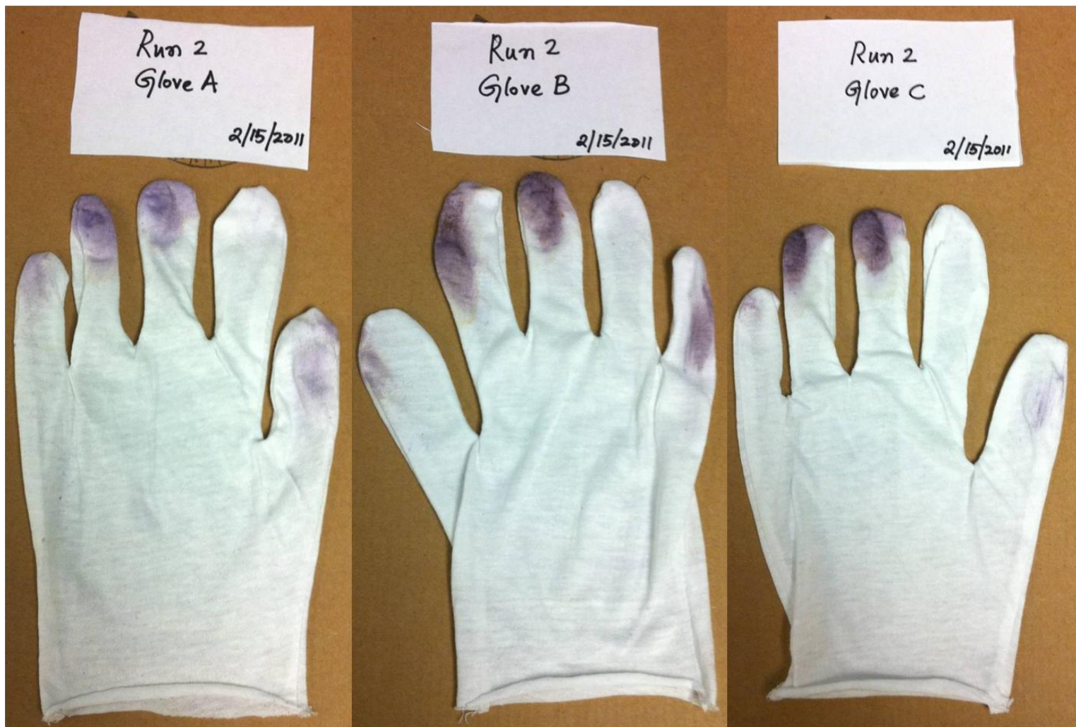
Figure 4.8: Cotton Gloves Show Indicator Dye (Contact) on Fingers After “Run 2” Pass on Turf Using the BCTU
