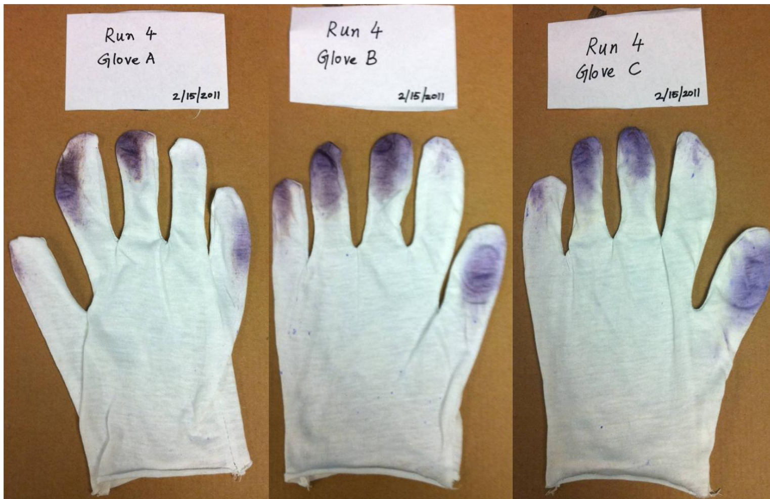
Figure 4.10: Cotton Gloves Show Indicator Dye (Contact) on Fingers After “Run 4” Pass on Turf Using the BCTU
