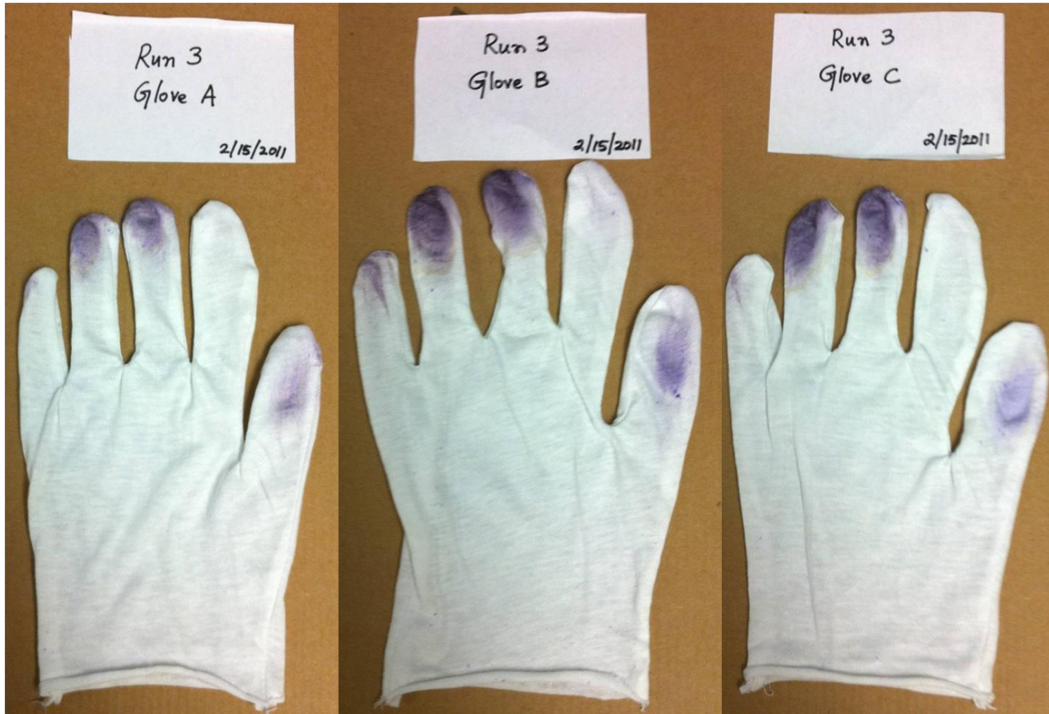
Figure 4.9: Cotton Gloves Show Indicator Dye (Contact) on Fingers After “Run 3” Pass on Turf Using the BCTU
