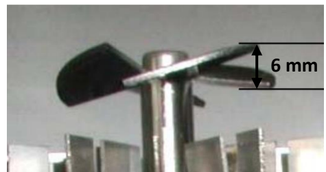
Figure 16. Correct stirrer pitch + blade thickness.
