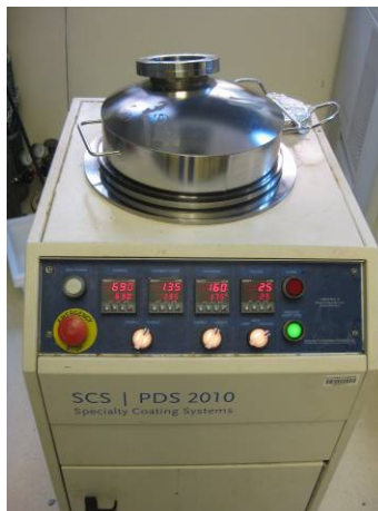
Figure 24. Parylene Coater from Specialty Coating Systems
