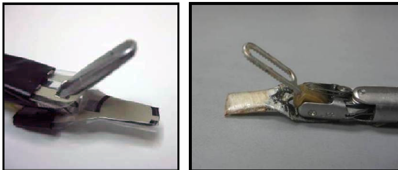
Figure 23. Improved sensor mounting process, (Left) on a laparoscopic instrument (Right) On a da Vinci Grasper
