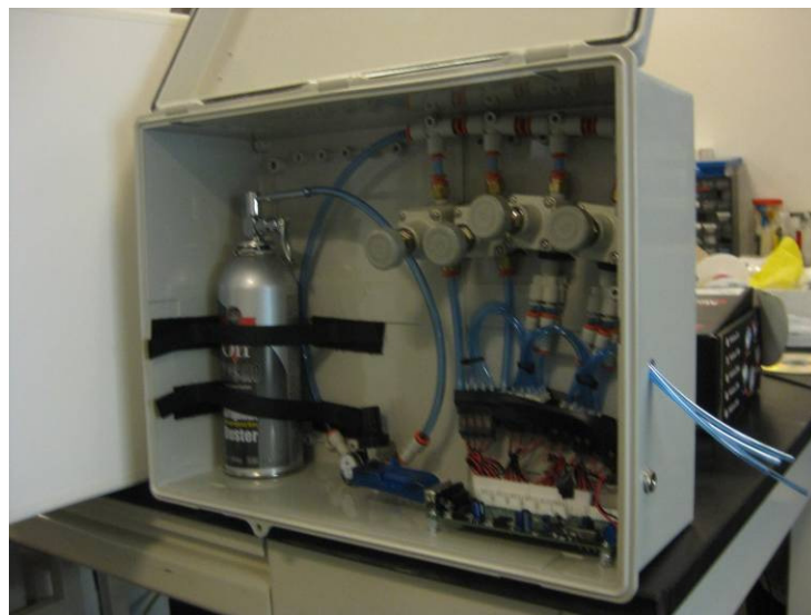
Figure 58. Tactile feedback system mounted in a plastic project enclosure.
