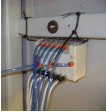
Figure 35. (Left) SMC ITV-0010 pressure regulators mounted in the da Vinci Surgical System (Right) Functional Block diagram of initial pneumatic system
