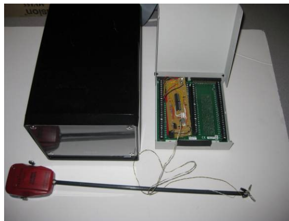
Figure 104. Initial version of Remote Tactile feedback system with Data Acquisition Board and Shuttle PC connected to Internet.
