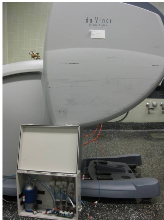
Figure 65. The receiver circuit and pneumatic system housed in a plastic enclosure and positioned near the da Vinci console, along with a back-up air canister.
