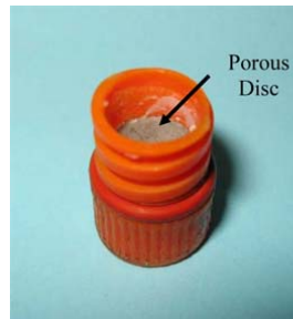
Figure 2.5 Fluid collection system for permeameter (top). Specimen holder close up (bottom)
