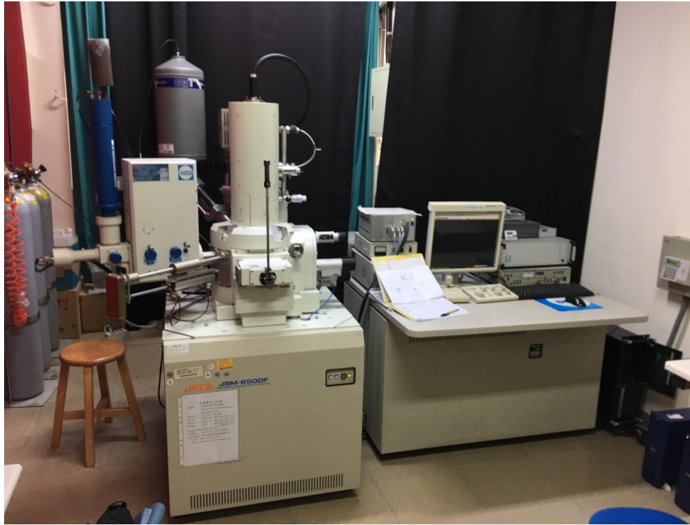
Figure 1-7 The scanning electron microscopy (Model JEOL JSM-6500 F) at NCTU.
