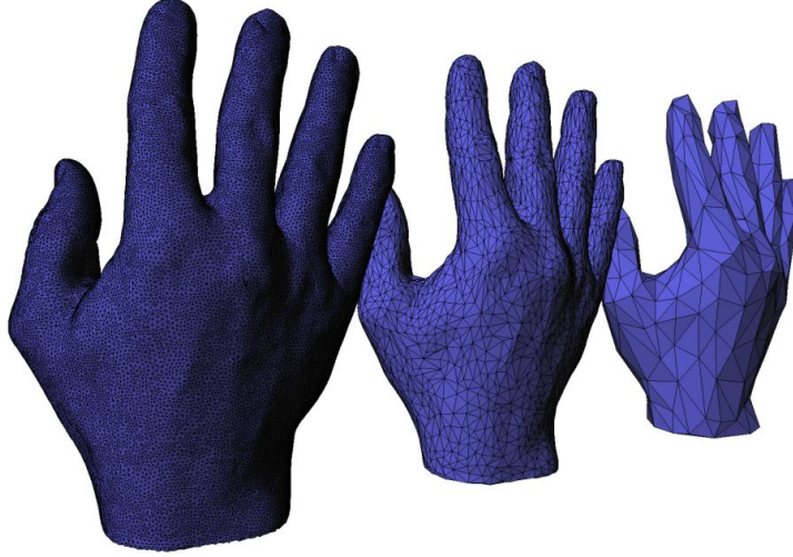
Figure 5.2: Surface mesh simplification algorithm applied to a mesh with different simplification levels [5].
