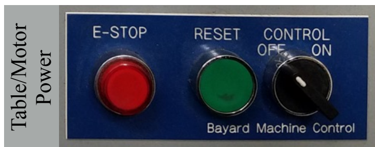
Figure 2.9: The power controls for the libration experiment.
