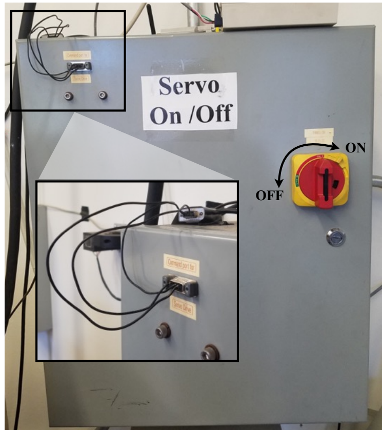
Figure 7.33: The servo drive front panel with the main power switch located on the right side. An RS232 plug is also located on the top left of the front panel and shown inset. The RS232 cable runs from the fumehood computer where the rotation is controlled to the servo drive box where the servo drive is kept.
