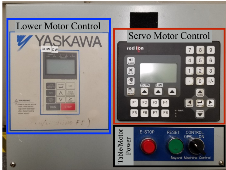
Figure 2.8: Control console for the librational forcing experiment. The green outlined region is the control pad for the lower table that provides a constant rotation rate. The red outlined area is the control pad for the oscillating servomotor. The lower controls outlined in black are the main power switches for the entire device.
