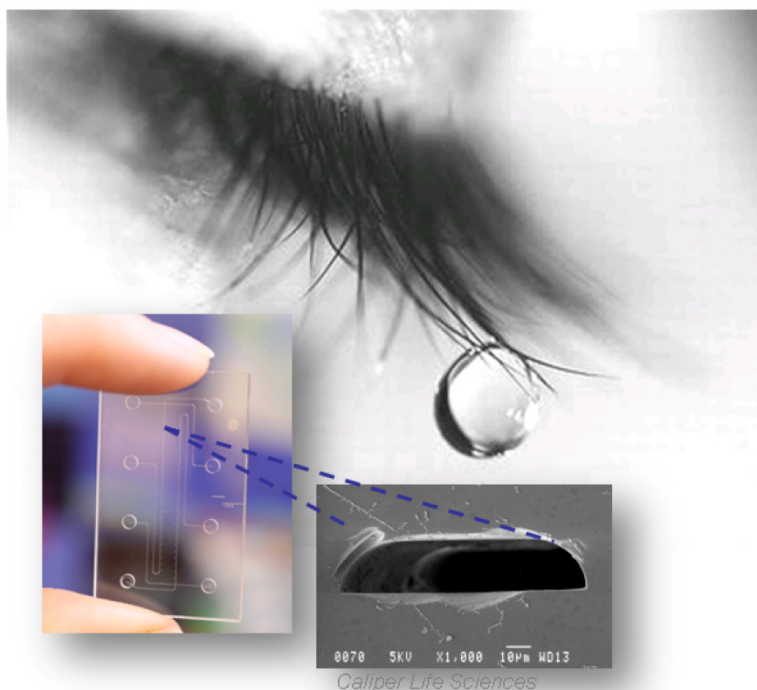
Figure 19. The small sample requirements of microfluidic homogeneous immunoassays make them well-suited for human tear protein analysis. A picture of the microfluidic chip used in this work is shown as well as a scanning-electron-microscope image of the channel cross-section, courtesy of Caliper Life Sciences. Image of tear is from wallpaperswide.com 147
