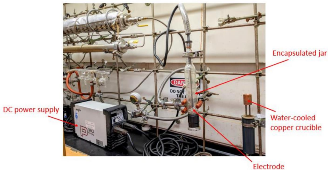
Figure 1.6 Fokwa Lab Arc melting apparatus. 9
