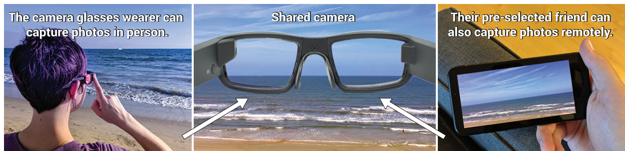
Figure 4.2: Overview. Friendscope’s key innovation is its shared camera , which enables wearers to share control of their camera directly with a pre-selected friend so that both of them can capture photos/videos. The friend is therefore able to receive photos/videos on demand, anytime, as if they are viewing the experience live.
