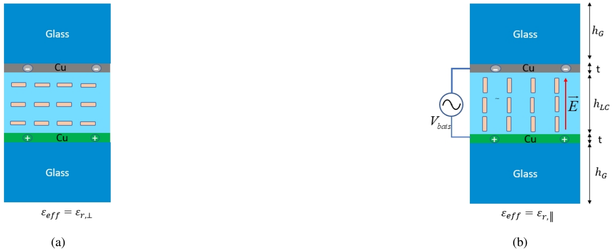
Figure 2.2: Variable capacitance shown in Figure 2.1c, is created by a sandwiched LC material between two electrodes for applying electric field. The effective permittivity of the LC material is changed from (a) when there is no external bias voltage, to (b) when saturated bias voltage is applied.
