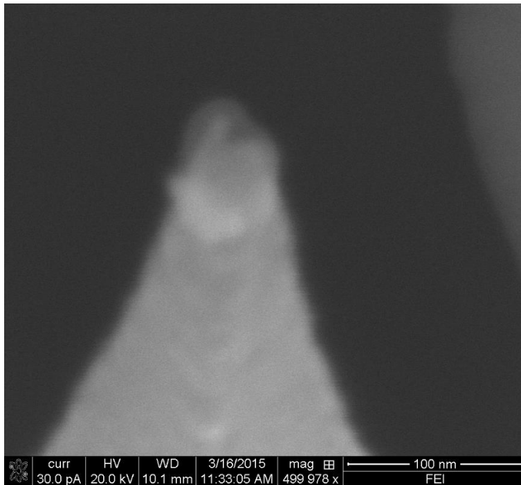
Figure 58 SEM image of Au nano rod attached to the end of the tip
