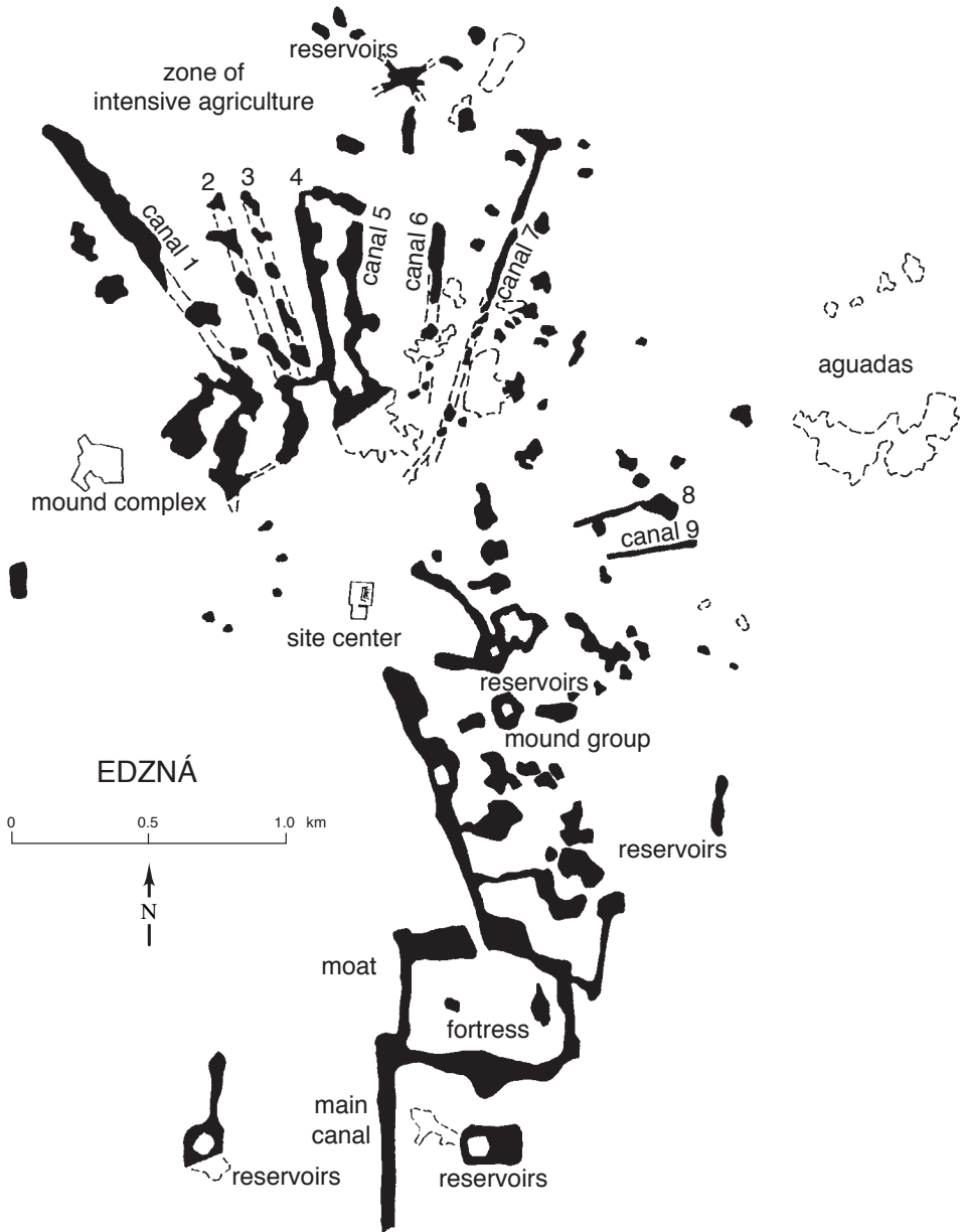
Figure 9.8. The Maya site of Edzná in Mexico features an impressive water-storage system of canals, reservoirs, and a moat (redrawn from Matheny 1978:Figure 10.8).
