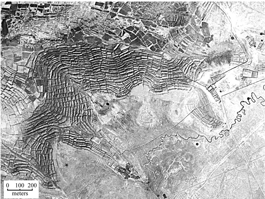
Figure 13.9. An integrated, engineered landscape of terraces (upper left) and raised fields (lower right). The landscape capital includes construction of many linear kilometers of terrace and field-boundary walls, movement of massive volumes of earth, and reworking of soil horizons to a depth of 1 meter or more.
