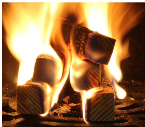
Figure 8.1: Wood configuration consisting of 5 sticks stacked in a slightly askew pyramid used for the BDS LE trials as viewed from the firebox opening.
