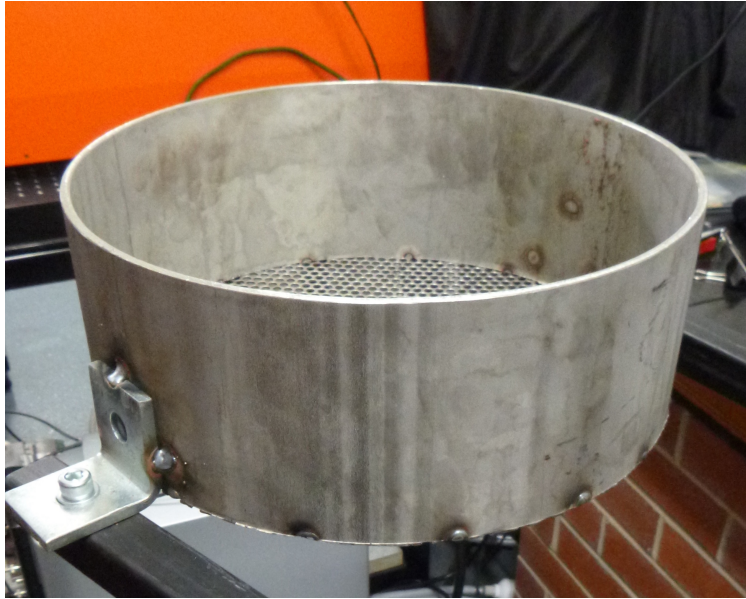
Figure 2.6: Picture of the sieve particle seeder without lid and fine mesh insert. The seeder was mounted using L-brackets to identical lever arms. The seeder could then be vibrated above the measurement region to introduce particles.
