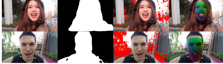
Figure 3.4: Our selfie video dataset. From left to right: color frame, ground truth foreground mask, background feature points, face mesh.
