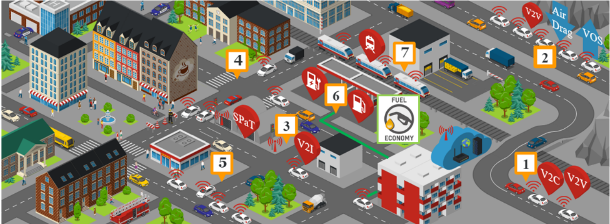
Figure 1.1: Cartoon illustrating a variety of intelligent transportation systems enabled by connected and automated vehicles (CAVs). (1) Longitudinal motion control with V2C and V2V, (2) compact platooning, (3) enhanced approach and departure to signalized intersections, (4) shared perception, (5) coordinated movements, (6) eco-routing, and (7) virtual coupling for railway (Created on https://icograms.com ).
