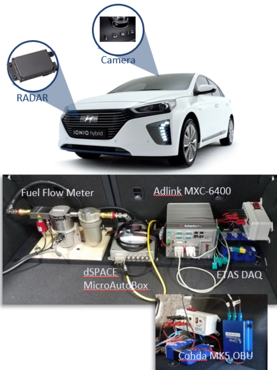
Figure 2.5: Hardware instrumentation for connected and automated vehicles
