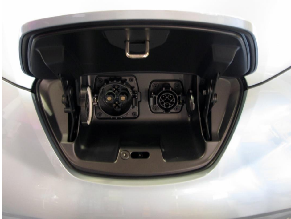
Figure 11. PEV charging connectors for level 3 on the left and levels 1 and 2 on the right, from U.S. Department of Energy [129]
