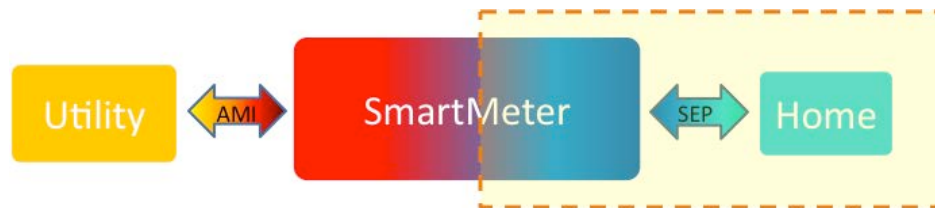
Figure 1. Relationship between utility, meter, and home with AMI and SEP
