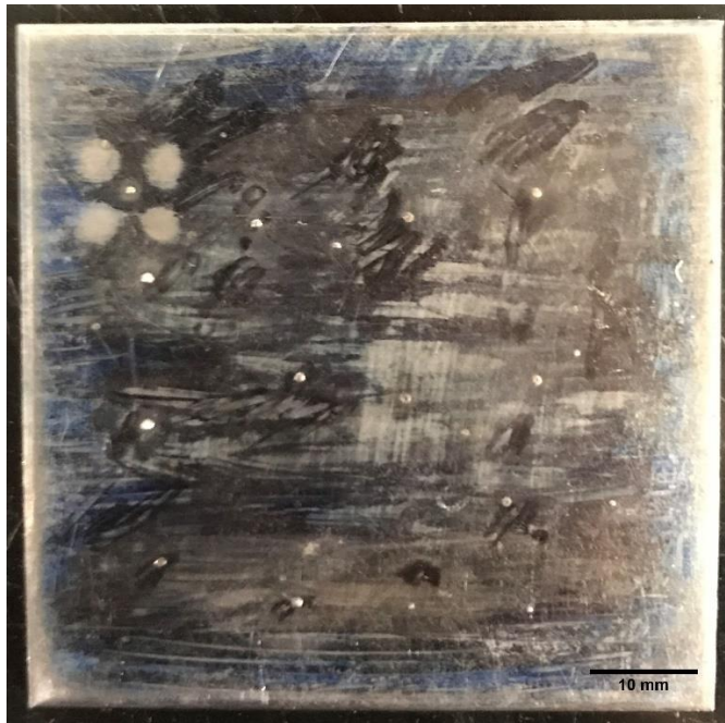
Figure 3.3. Alignment test piece coated with black Sharpie and the resulting powder dispersion pattern with aligned laser mark.
