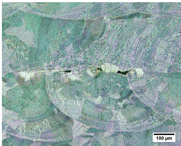
Figure 2.9. Lack of fusion porosity found in sample from 105° build.
