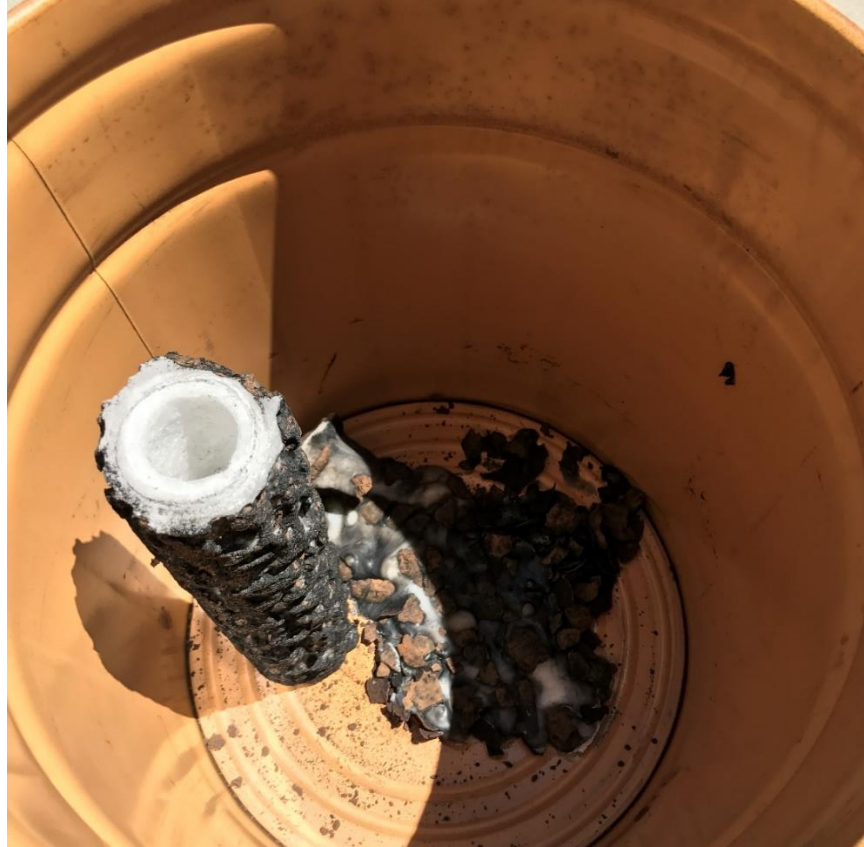
Figure 3.10. Burned filters after immediate exposure to air. The filter on the left is partially melted while the filter on the right melted down completely.
