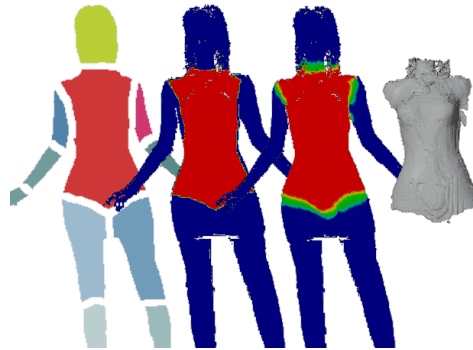
Figure 3.3: Projection-based mesh segmentation. Left to right: 2D segmentation, back-projection assignment, smoothing with diffusion, final segmentation.
