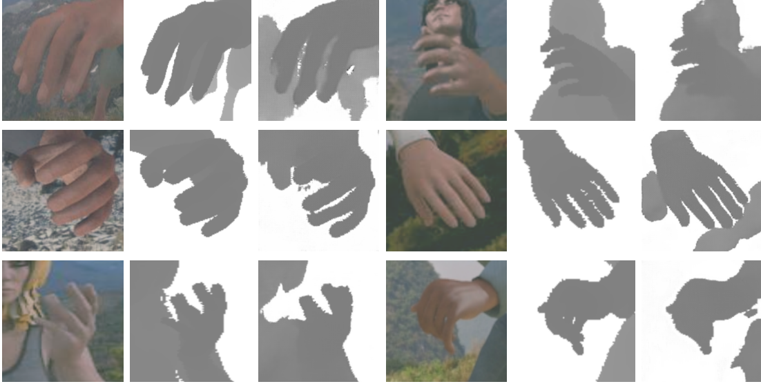
Figure 3.7: Comparison between the generated and ground-truth depth maps on the RHD dataset. The first and fourth columns show the RGB images. The second and fifth columns display the real depth maps. The third and sixth columns give the generated depth maps.
