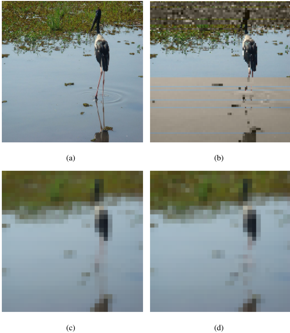
Figure 5.3: Visualization of AdaSkip-based subsampling. (a) The original 512 \times 512 image; (b) the output of the AdaSkip algorithm, where the greyscale parts are rows sampled with s_l = 8 and the colored part are rows sampled with s_h = 4 ; (c) 32 \times 32 output images from two-step subsampling with s = 4 and bilinear resampling; (d) 32 \times 32 images obtained by bilinear resampling the output in (b).
