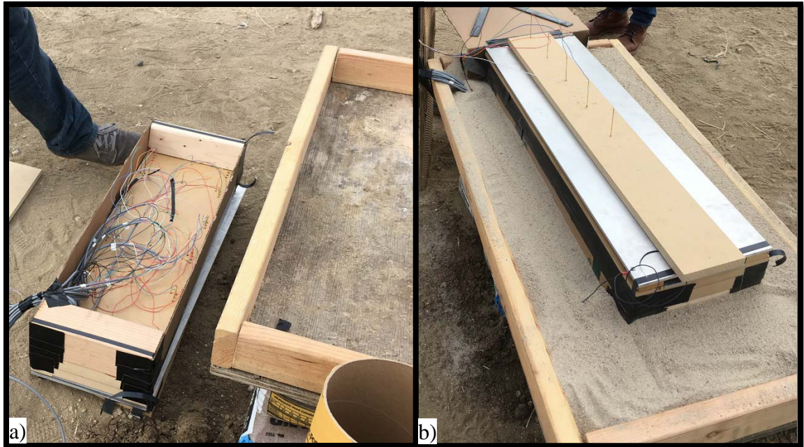
Figure 3-8: Welding anvil, used for tests. a) Tray and underside of sample frame, showing TOA pin connections, to be filled with moist sand. b) Filled tray and placed sample awaiting explosives.
