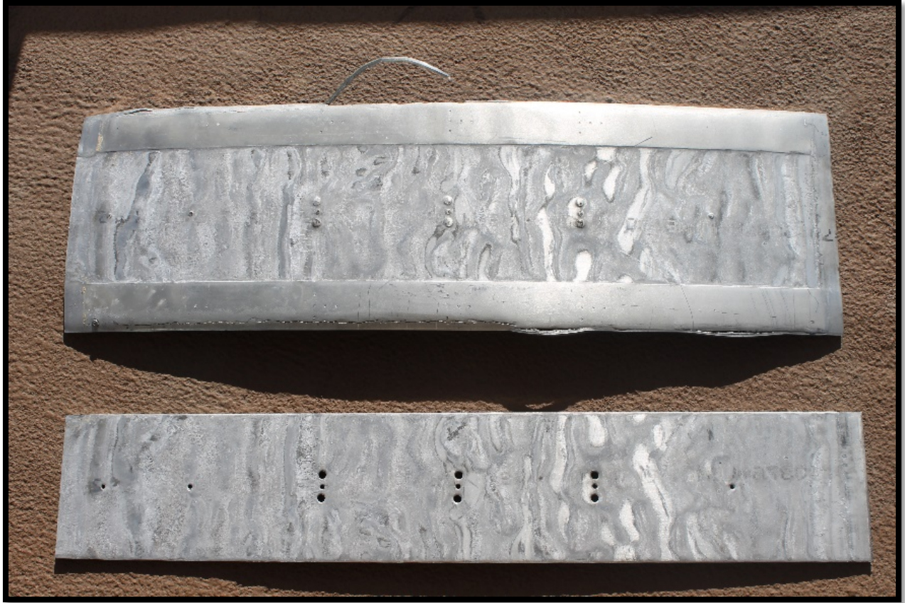
Figure 3-25: 0.5°, non-annealed, make-up test that failed to weld
