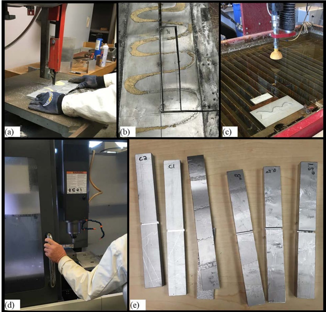
Figure 4-8: Fabrication of tensile shear specimens. (a) & (b) Band saw cuts to rough dimensions out of weld specimens. (c) Water jet cuts from control plate. (d) CNC milling to final dimensions. (e) Final specimens, showing one of the 2.5° specimens that failed during fabrication.
