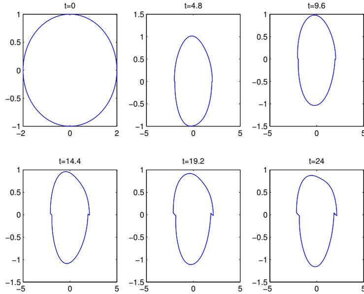
**Figure 6.16:** Solution of Geometric Airy curve flow on  $\mathbb{R}^2$  with initial data  $\gamma_0 = (2 \cos(2x), \sin(2x))$
