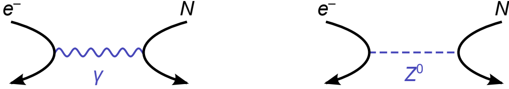
Figure 1.1: Feynman diagrams for two electron-nucleon radiative processes: (left) one governed solely by electromagnetic processes and (right) a second one involving exchange of the weak neutral gauge boson Z_0 .
