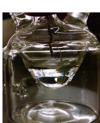
Trichel pulse discharge (Negative polarity, moderate applied voltage)
