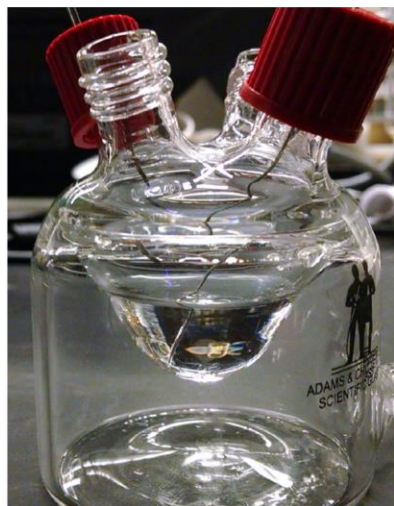
Streamer discharge (Positive polarity, lower applied voltage)
