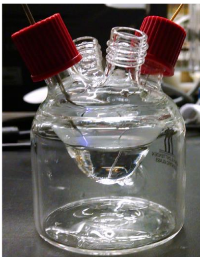
Transient spark discharge (Positive polarity, higher applied voltage)
