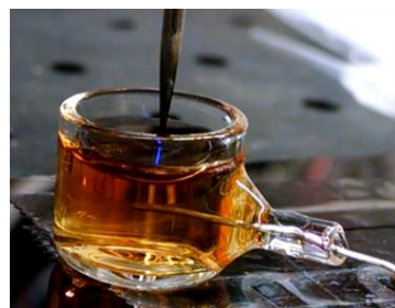
Thimble cell: SS anode, custom borosilicate vessel ( OD = 15\ \text{mm} , ID = 13\ \text{mm} , h = 12\ \text{mm} ) with Pt lead
