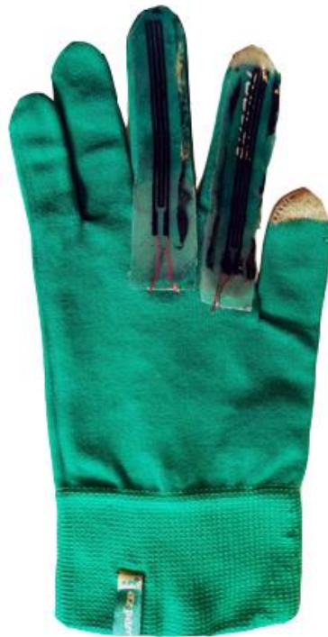
Figure 2.2 Soft Strain Sensors mounted on the glove
