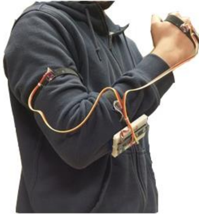
Figure 3.2 Mounting IMU using velcro
