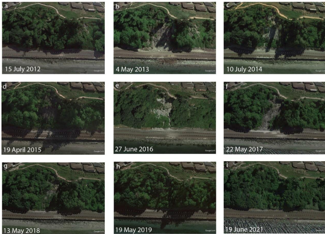
Fig. 3.6 | Images from Google Earth showing the changes in tree cover at LS due to landsliding and subsequent vegetation regrowth between 2012 and 2021.
