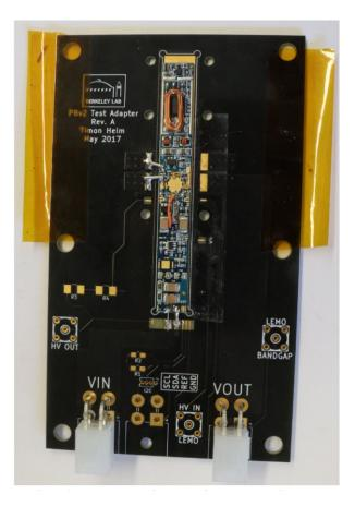
Figure A.4: Single power board test adapter.
