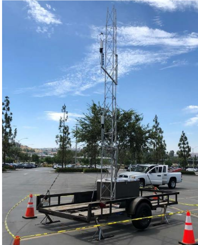
Figure 3-6 Upwind meteorological measurement site containing two 3-D sonic anemometers mounted at heights of 3 m and 5 m.
