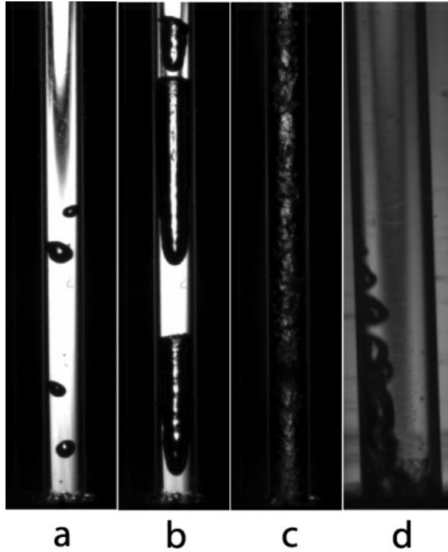
Figure 4.2: Flow regimes observed in the present study: (a) bubbly, (b) slug, (c) churn, and (d) tip evaporation.
