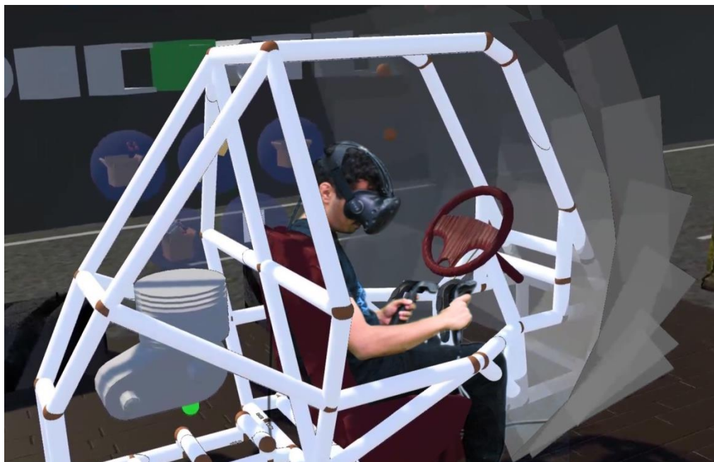
Figure 32. Ergonomic analysis of occupant package using maximum reach envelope
