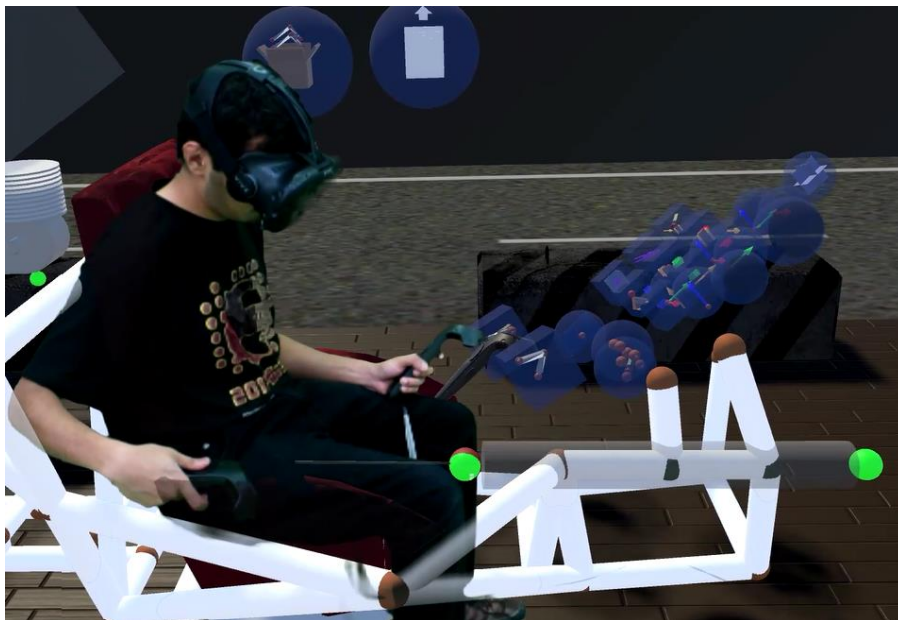
Figure 29. Virtual reference cylinder to aid in modeling set of collinear points
