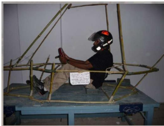
Figure 9. Ergonomic Analysis Mockup for the finalized design concept
