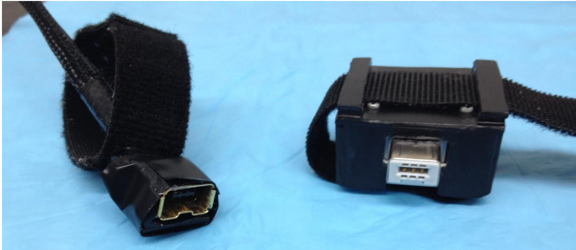
Figure 1.10: Fully Constructed Custom Wii Motion Plus Motion Sensor and Cable
