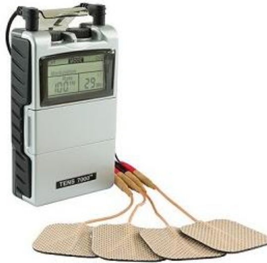
Figure 2.1: Unmodified TENS7000 Unit with Leads and Surface Electrodes
