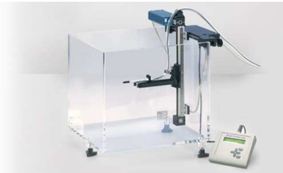
Figure 26. Water Phantom 1-Dimension (WP1D). Photo courtesy of IBA Dosimetry, WP1D manual.
