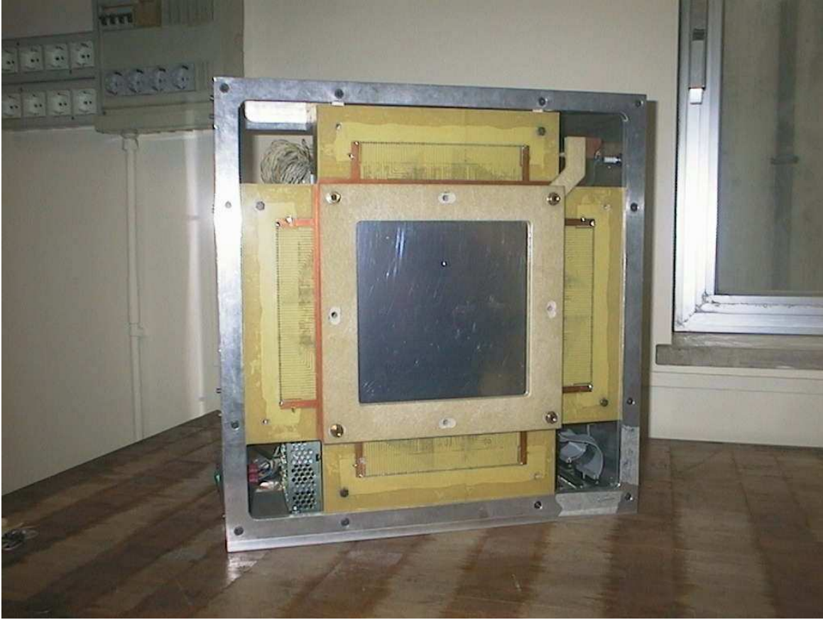
Figure 4. Pixel Ionization Chamber (PXC). Presented from Cirio et al.
