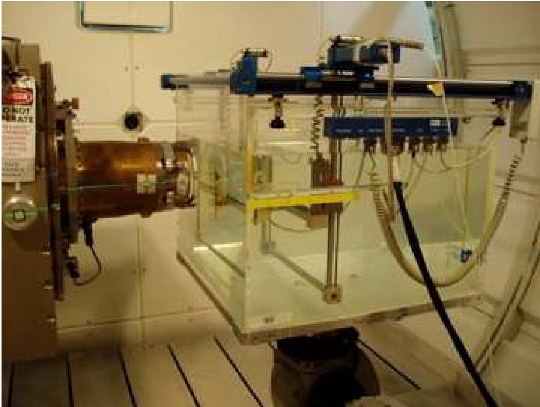
Figure 2. Water phantom, Markus chamber setup in gantry room.
