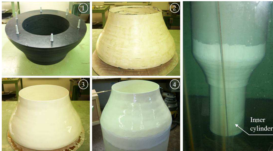
Figure 4.2: Fabrication of the Berkeley-Wedge bottom shape of the floater and close-view of bottom installed in wave-tank (right)
