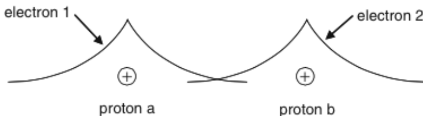
Figure 2.2: The hydrogen molecule consists of two protons, each with a bound electron. The protons are sufficiently close so that the electronic wave functions overlap.
