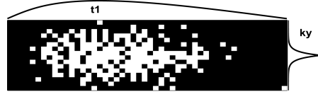
Figure 5.9: NUS mask used to prospectively NUS the k_y - t_1 plane 4X in Figures 5.7 and 5.8.
