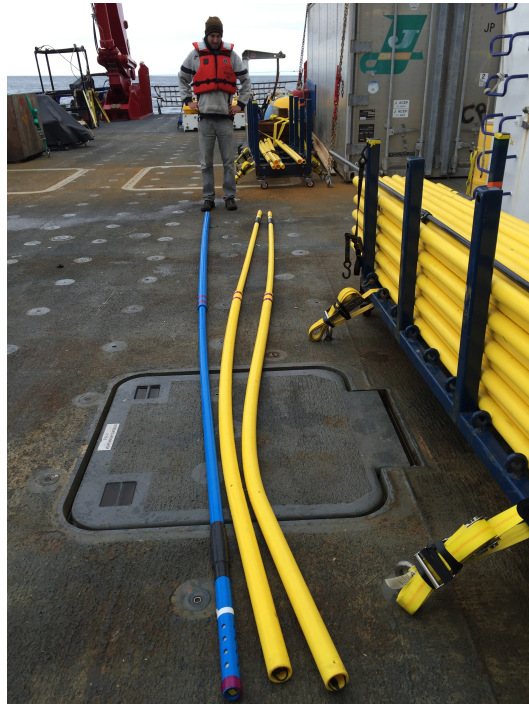
Figure 3.9: Bent electrode arms on station F17. Image courtesy of Kerry Key.
