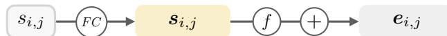
Figure 6.6: A diagram that shows the steps to make an utterance vector e_{i,j} speaker-dependent. A linear projection (FC stands for the fully connected layer) is performed to create a speaker embedding s_{i,j} , and the speaker embedding is added to the existing utterance vector after an activation function. The size of the speaker embedding is the same as that of the utterance vector e_{i,j} .
