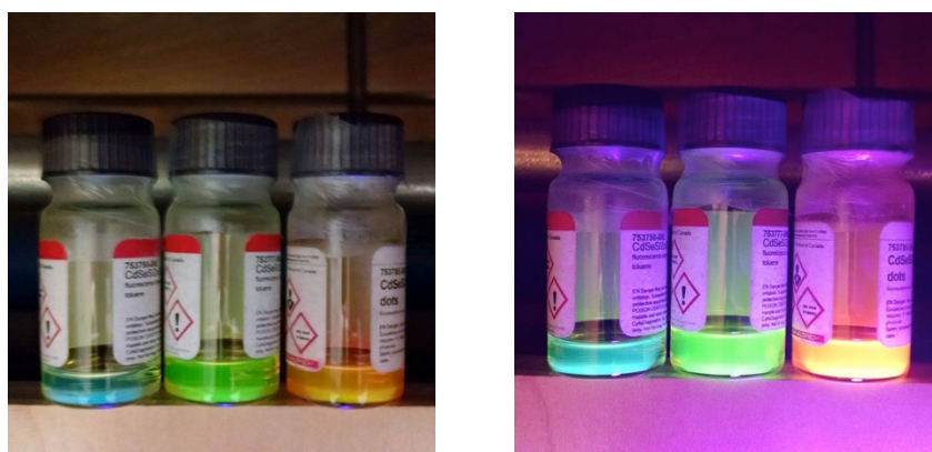
Figure 3.3 Pictures demonstrating the tunability of QD emission color with regards to size under normal light (left) and UV light (right). As QD size increases from left to right, emission wavelengths are 490 nm, 530 nm, and 580 nm.
