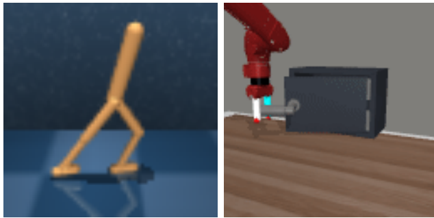
Figure 20: Our image-based environments: The observations are 64 \times 64 and 128 \times 128 raw RGB images for the walker-walk and sawyer-door tasks respectively. The sawyer-door-close environment used in in Section 5.2.5.1 also uses the sawyer-door environment.
