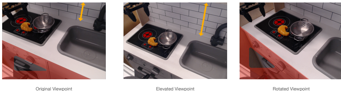
Figure 50: Sample observations from different camera viewpoints, only used during fine-tuning. Left: the original camera viewpoint found in Figure 49. Middle: an elevated camera viewpoint where the robot and camera have been raised 7 cm. Right: a rotated camera viewpoint where the kitchen has been slightly translated and rotated 15 degrees counterclockwise relative to the camera and robot.
