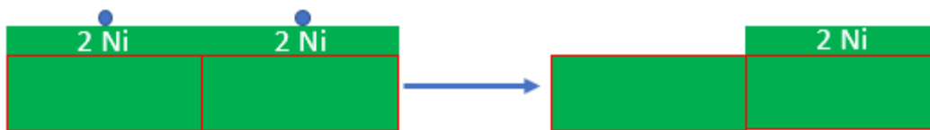
Figure A.1 the layer-by-layer removal model on oxygen activated Ni surface at \frac{1}{2} ML coverage. Two copies of the activated surface are needed to remove one layer on a single copy, leaving the other copy unetched.
