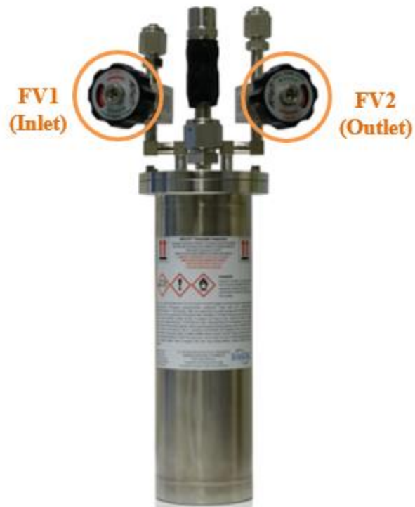
Figure D.4 Hydrogen peroxide vessel.
