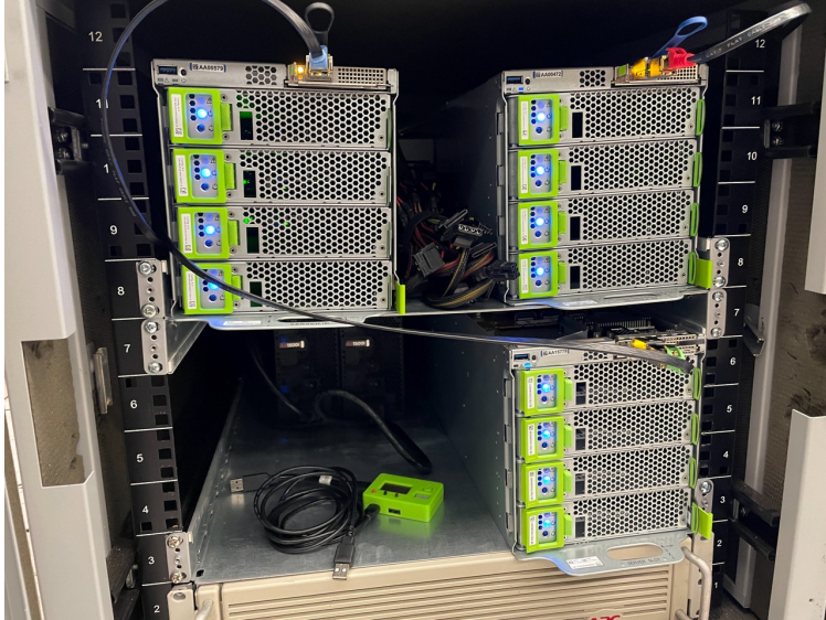
Figure 5.12: 12 nodes (3 sleds \times 4 nodes) of Yosemite V3 Open Compute Project (OCP) used for experiments. These servers are representative of datacenter racks.
