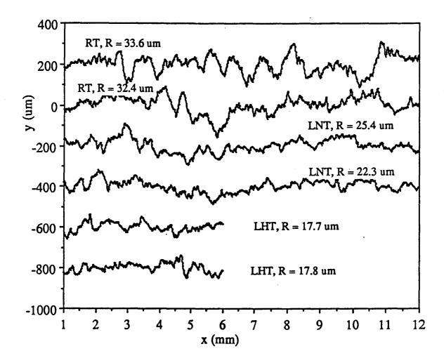
Fig. 4: Profilometer line scannings of the fatigue fracture surfaces of the specimens that were fatigue tested at room temperature (RT), liquid nitrogen temperature (LNT), and liquid helium temperature (LHT). Cracks propagated from right to left, the roughness parameter R is defined in the text.
