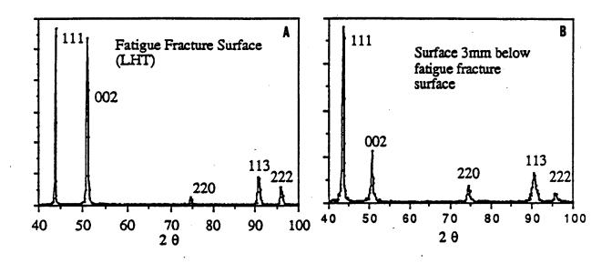
Fig. 5: X-ray diffraction data of (a) fracture surface of the fatigue specimen tested at liquid helium temperature (LHT) and (b) the surface 3mm below the frature surface.
