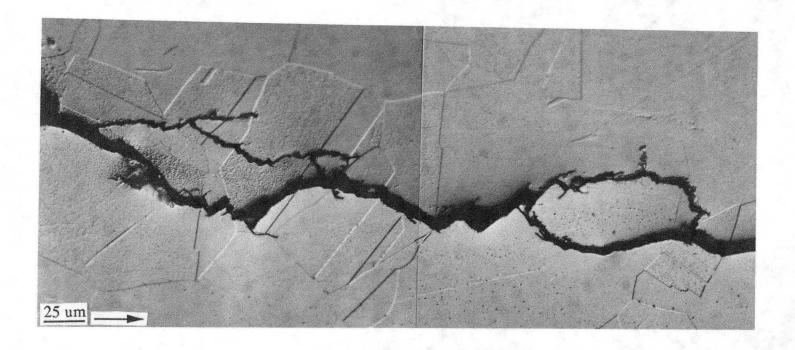
Fig. 2: Optical micrograph of the fatigue crack profile of the specimen tested at liquid helium temperature.
