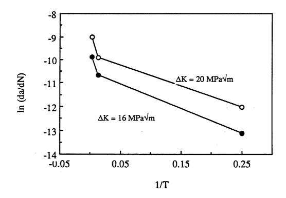
Fig. 6: Two plots of  $\ln(da/dN)$  vs. 1/T at  $\Delta K = 20$  and 16 MPa- $m^{1/2}$ .
