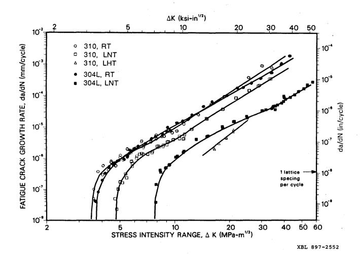
Fig. 1: Fatigue crack propagation curves of 310 and 304L austenitic stainless steels at room temperature (RT), liquid nitrogen temperature (LNT), and liquid helium temperature (LHT).
