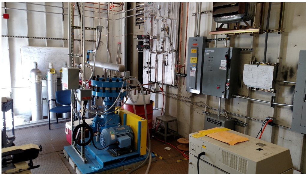
Figure 6.4.3: Fluitron 100 slpm all-metal single-stage diaphragm compressor operating as part of SLAC System Test.
