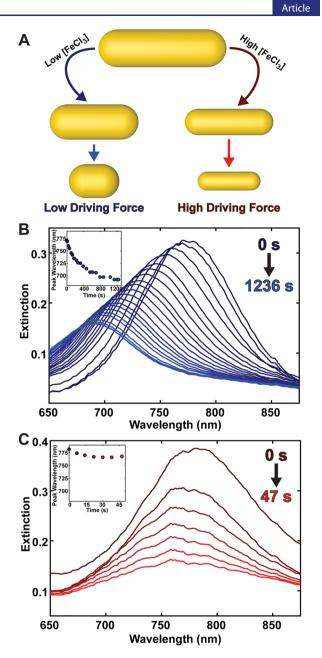
**Figure 5.** Ex situ low-driving-force and high-driving-force oxidative etching of gold nanorods. (A) Schematic of low-driving-force etching from the tips of the nanorod and high-driving-force etching maintaining the aspect ratio. (B) Extinction spectra while etching in a low-driving-force regime. The inset shows the LSPR blue shifting during etching. (C) Extinction spectra while etching in a high-driving-force regime. The inset shows the LSPR staying relatively constant.
