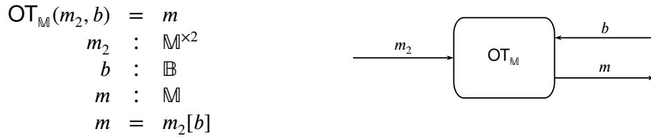
Figure 5.1. A naive OT functionality: the receiver gets the selected message m = m_2[b] , and the sender does not get anything at all.
